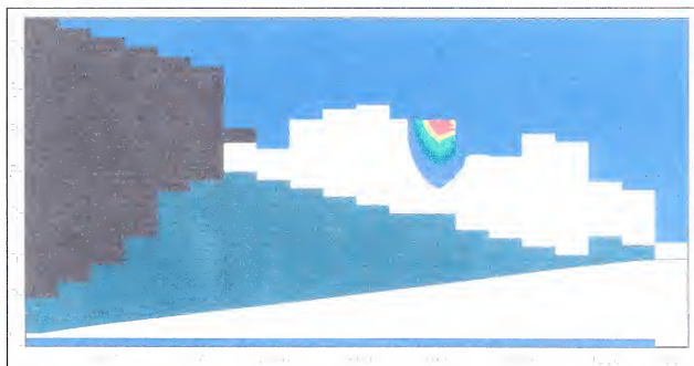
Figure 22 Leachate plume of CHCs after 10 years. Upper image shows horizontal distribution while the lower image indicates vertical distribution. Concentrations measured in mg/L.
